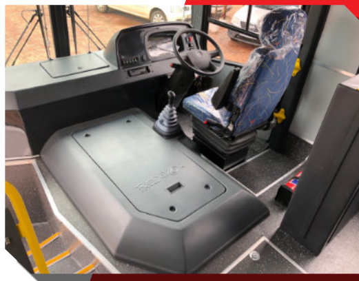
Modern G.R.P dashboard, with sound & heat insulation built-in
