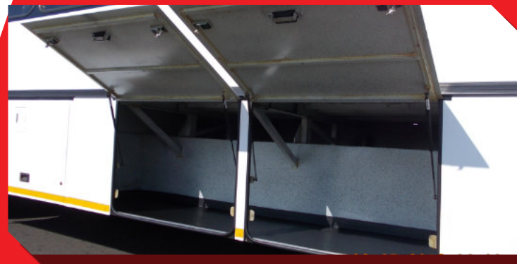
Maximum luggage lockers with locker Space across the chassis - Max capacity of approximately 5m 3
