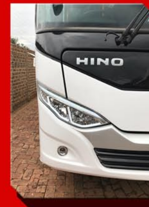
One piece cluster headlight with LED daytime running lights and LED spot lights
