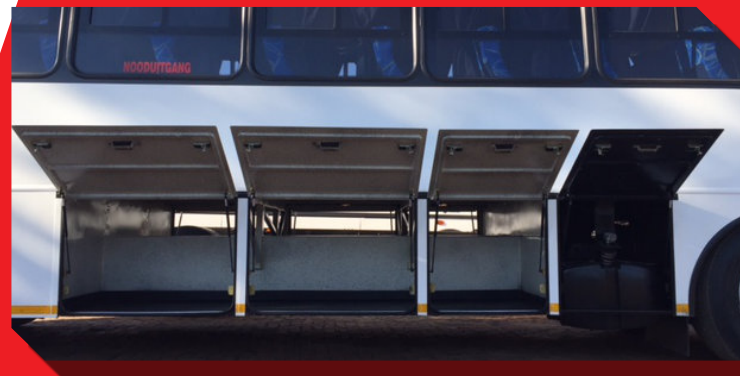
Maximum luggage lockers with locker Space across the chassis - Max capacity of approximately 6m 3
