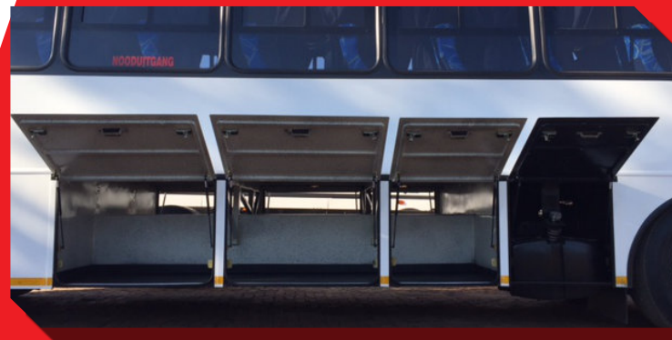
Maximum luggage lockers with locker Space across the chassis - Max capacity of approximately 6m³
