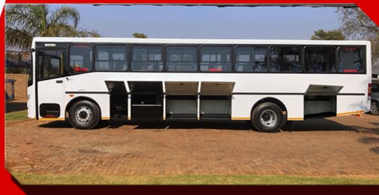
Maximum luggage locker with locker space across the chassis - Max capacity of approximately 6m 3
